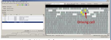
Identify driving cell of suspect net(s) and via(s)
